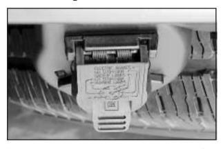
Your vehicle may be equipped with the seven-wire trailer towing harness. This harness has a seven-pin universal heavy-duty trailer connector that is attached to a bracket on the hitch platform. The seven-wire harness contains the following trailer circuits:
